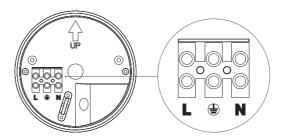
Fit the head unit to the base plate ensuring that the three Quick-Connect pins and mounting legs are lined up. Re-fit the head unit screws. **Caution: Do not over tighten head unit screws.**
