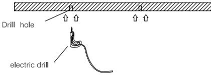
2. Fix the surface mount clip to the ceiling.
