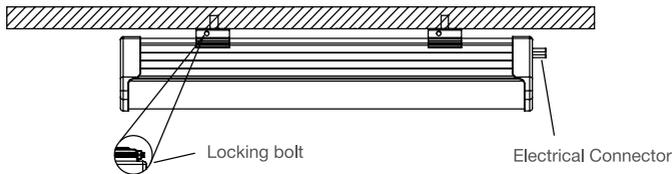
4. Repeat the above for subsequent Link Battens and attach connection clip and tighten locking bolt. Attach power cable to one side of the run length and end cap to the other. Turn on power.
