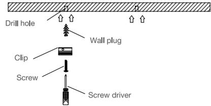
3. Attach the batten to the clips, fix the screw, and then insert electrical connector on the end of light as required. Tighten the locking bolt.
