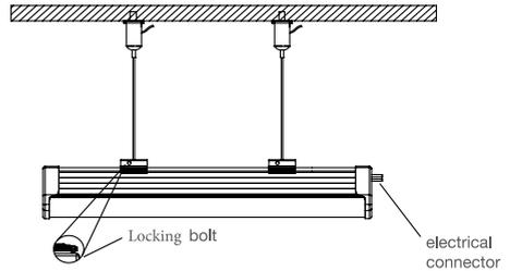
5. Repeat the above for subsequent Link Battens and attach connection clip and tighten locking bolt. Attach power cable to one side of run length and end cap to the other. Turn on power.
