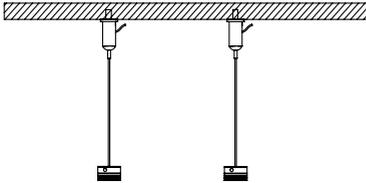
4. Attach the batten to the clips and tighten the locking bolt. Attach electrical connector at the end as required.
