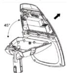
6. Wire the incoming AC wires into the terminal block ensuring that the wires are in the correct positions. Ensure that the wires are tightened securely.
