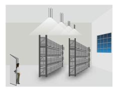
When the ambient light level is below the selected **daylight threshold** the [SMARTBAY] will turn on when motion is detected.
