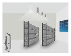
When no movement is detected after the selected hold time, light will dim to the selected standby dimming level.
